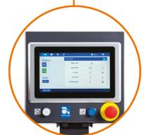
AutoTouch™ Control Screen accesses operator tutorials, help system, on-board diagnostics, and performance monitoring
