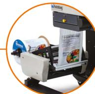
Multi-position unwind with tension control simplify changeover
